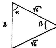
$$\begin{aligned} \cos \alpha &= 1/\sqrt{6} \\ \alpha &\approx 65.9^\circ \\ \beta &\approx 48.2^\circ \end{aligned}$$
